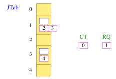
Thread 0 is running, thread 1 could run, threads 2 and 3 wait for the termination of 1, and thread 4 waits for the termination of 3.
