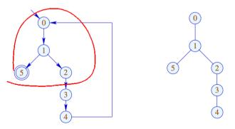
Here, the complete block between back edge and conditional jump should be duplicated.
