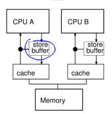
put each write into a store buffer and trigger fetching of cache line **Store Buffers**
