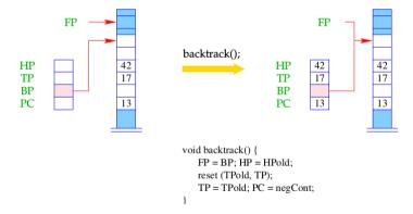
where the run-time function reset() undoes the bindings of variables established since the backtrack point.
