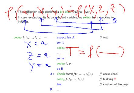
The instruction check i checks whether the (unbound) variable on top of the stack occurs inside the term bound to variable i.
